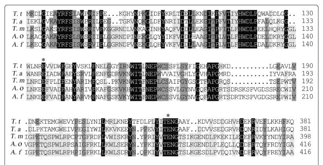
**Figure 1 Multiallignment of BGL with some GH1 family members.** Sequence alignment was performed by using Clustal X2.0. The active sites are indicated as\* on the top of the alignment. *T. t. T. thermosaccharolyticum* DSM 571 (YP\_003852393.1), *T. a: Trichoderma atroviride* (EHK41167.1), *T. m: Thermotoga maritima* (Q08638.1), *A. o: Aspergillus oryzae* (BAE57671.1), *A. f: Aspergillus fumigatus* (XP\_752840.1).
