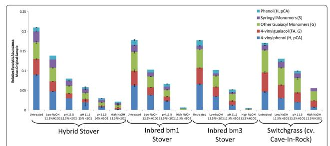
**Figure 3 Pools of aromatic pyrolysis products as a function of biomass source and pretreatment.** The data were normalized to the mass of the original sample based on the quantified mass loss during pretreatment and provide an approximation of the relative abundance of the five pools of aromatics volatilized by pyrolysis.
