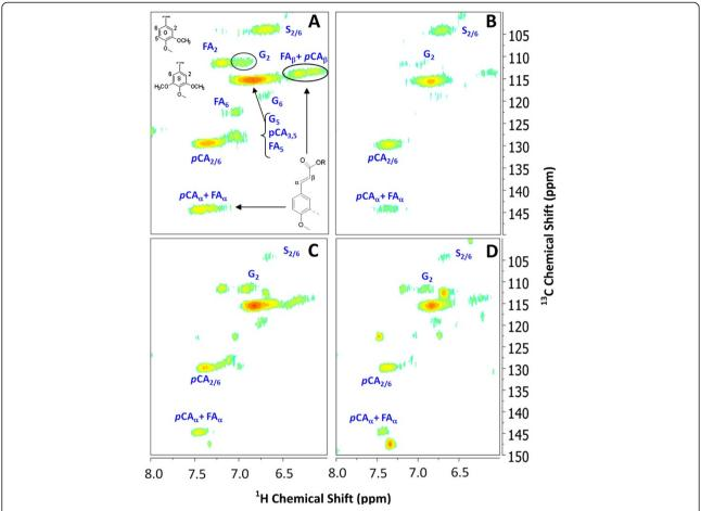
Figure 7 Aromatic region of <sup>13</sup> C-<sup>1</sup> H HSQC spectra of (A) untreated and (B) AHP pretreated hybrid corn stover and (C) untreated and (D) AHP pretreated inbred bm3 corn stover in perdeuterated pyridinium chloride/DMSO-d<sub>6</sub>.
