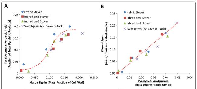
**Figure 4** Correlating pyrolytic yields of aromatics to Klason lignin. A comparison of all biomass types for all pretreatment conditions shows that the relationship between (A) aromatic pyrolytic yield *versus* Klason lignin and (B) the pyrolitic 4-vinylguaiacol as a proxy for cell wall ferulates *versus* Klason lignin with both normalized to the mass of the untreated sample to indicate the amount of material removed from the cell wall.
