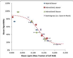
Figure 1 Correlating Klason lignin content of the cell wall to glucan digestibility for all pretreatment conditions and biomass types.
