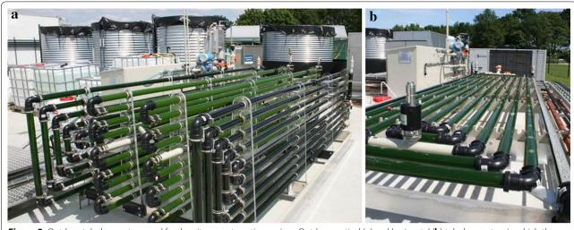
Figure 3 Outdoor tubular reactors used for the nitrogen-starvation regime. Outdoor vertical (a) and horizontal (b) tubular reactors in which the nitrogen-starvation regime was performed.
