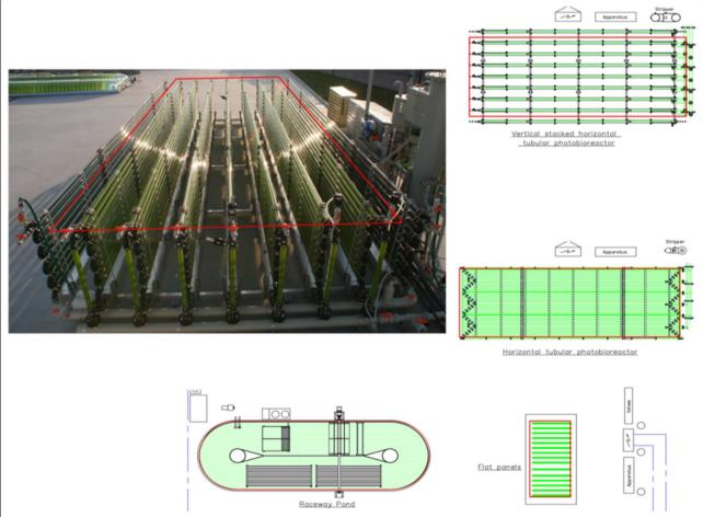
**Fig. 5** Ground area considered for calculation of areal productivity and photosynthetic efficiency for each photobioreactors. *Top left* photograph of vertical tubular photobioreactor with area considered as ground area indicated by *red lines*
