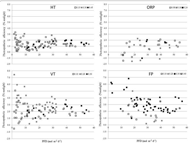
**Fig. 3** Influence of daily photon flux density on photosynthetic efficiencies on sunlight for the different photobioreactors. For the horizontal tubular photobioreactor (HT), open raceway pond (ORP), vertical tubular photobioreactor (VT) and flat panel photobioreactor (FP). The *different colors* of the *squares* indicate different dilution rates applied to each different photobioreactor
