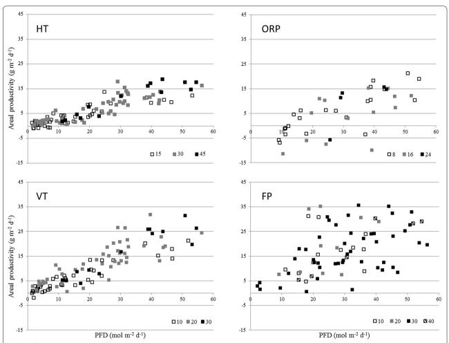
Fig. 1 Influence of daily photon flux density and dilution rate on areal productivity. For the horizontal tubular (HT), open raceway pond (ORP), vertical tubular (VT) and flat panel (FP). The different colors of markers indicate the different dilution daily rates
