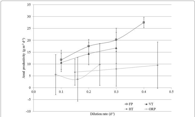
**Fig. 2** Average areal productivity versus dilution rate for each photobioreactor. Flat panel (FP), vertical tubular (VT), horizontal tubular (HT) and open raceway pond (ORP). Average areal productivity was calculated over a number of days for each dilution rate; FP; 6, 3, 40, 4, VT; 18, 39, and 14, HT; 19, 38, and 11, ORP; 22, 13, and 5
