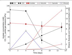
**Fig. 2** Standard production profile of the co-culture in non-shaking conditions. On all data series, a standard deviation is displayed over duplicate experiments. *Solid* and *open circle* symbols represent *left* and *right y-axis*, respectively
