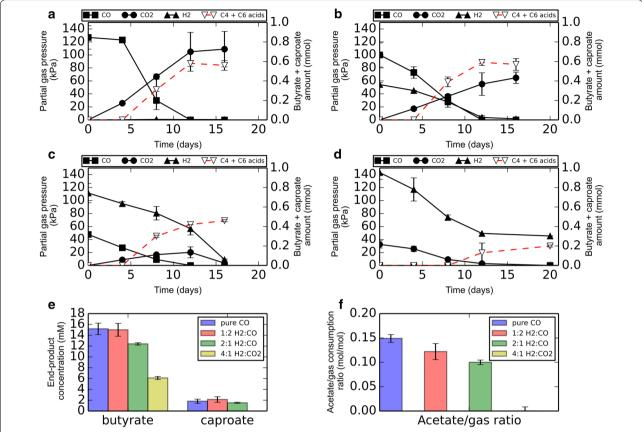
Fig. 4 The effect of  $H_2$ :CO ratio on the production profile of the co-culture. **a** Pure CO headspace. **b** 1:2 ratio of  $H_2$ /CO **c** 2:1 ratio of  $H_2$ :CO. **d**  $H_2$ /CO<sub>2</sub> headspace. **e** Product concentrations at the end of incubation. **f** Mole of acetate consumed per mole of gas  $(H_2 + CO)$  consumed. On all *graphs* a standard deviation is displayed over duplicate experiments. *Solid* and *open circle* symbols represent *left* and *right y-axis*, respectively
