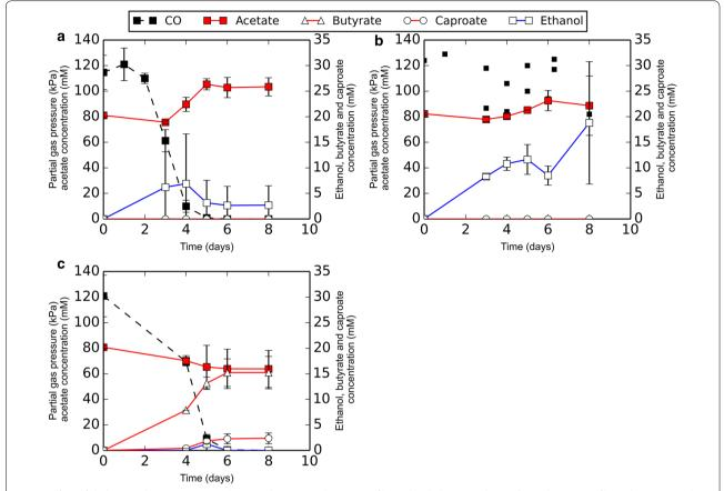
Fig. 5 Effect of shaking and CO pressure on the co-culture. **a** Production profile under shaking conditions. **b** Production profile with maintained CO pressure (>50 kPa), under shaking conditions. **c** Production profile after initial non-shaking incubation and subsequent transfer to shaking conditions (after t = 4). On all data series, a standard deviation is displayed over duplicate experiments. *Solid* and *open circle* symbols represent *left* and *right y-axis*, respectively
