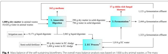
**Fig. 4** Mass balance of the self-sustaining biorefinery. The overall mass balance analysis was based on 1000 g dry animal wastes. *a* The mass balance for fungal fermentation was calculated based on 50 mL flask data. *b* The EC process used the mixture of fermentation effluent and liquid digestate to generate the EC water for the fermentation use
